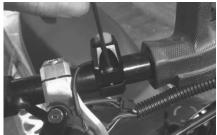
(6) Remove the clamp from the Munster reverse switch with an Alan key and install the switch on the handlebar in your desired position.
