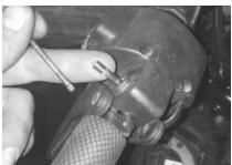
(3) Remove the pivot pin and sleeve from the throttle block. The throttle assembly should now split apart from the handlebar.
