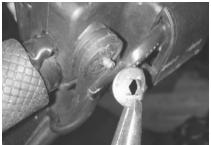
(2) Using small needle nose pliers, remove the pivot pin retaining clip from the bottom of the thumb throttle assembly.
