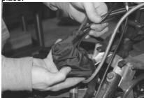
(6) With your new kill switch connected, cover up the harness plugs with the cloth boot and tuck them back into the machine. Put the hood back on (if it was taken off) making sure to connect all the harness plugs that were disconnected earlier. Fasten all hood bolts and rivets and install side panels.
