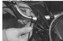
(8) Use zip ties to fasten the kill switch wires to the handle bar and you're done!
