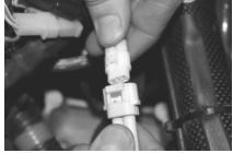
(5) Disconnect the plug connected to your stock kill switch and plug in the Munster kill switch in it's place.
