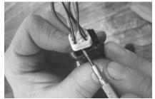
(4) Pull the rubber seal out and slide it back along the wires to give yourself enough room to pull the wires out individually.
