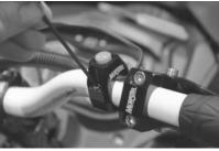
(6) Remove the clamp from the Munster kill switch with an Alan key and install the kill switch on the handle bar in your desired position. Route the
