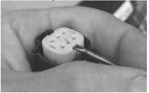
(5) Release the locking tabs holding the front cap on and pull the cap out until it stops. A second set of locking tabs prevent the cap from coming off. Pry back the second set of locking tabs to remove the cap completely. You should now be able to see all the tabs holding each terminal in and pry them back to remove them. Pull the wires through the rubber seal and backing plate of the plug connector.
