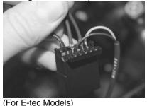
(15.1) Plug the pin connectors for the finger heater into the plug where the thumb heater was. The wires can be inserted in any order. Make sure they are inserted in the right direction. Flip the plug locking mechanism closed, making sure both locking tabs snap shut. Plug the connector plug back into the wiring harness.
