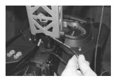
(11) Re-route the throttle cable through your riser so it can be installed in front of the handlebars. Keep in mind the cable must be clear of the riser cover when it is installed later. Make sure the cable housing is away from any pinch points. Check your steering for full range of motion making sure it doesn't put any tension or stress on your throttle cable housing.
