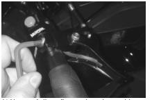
(18) Adjust finger throttle position for rider preference and tighten clamp bolts.
