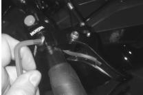
(10) Undo the clamp bolts on your new finger throttle using an Alan key. Route the wires from the heated grip through the slot in the throttle block. Clamp the finger throttle assembly to the handle bar and snug up the clamp bolts being sure not to pinch the wires.
