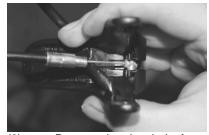
(2) Remove the pivot bolts from the thumb lever with an Alan key to detach it from the assembly. With the thumb lever off, pull the cable end out of the thumb lever by pulling on the cable housing. Try not to kink the cable while removing it from the lever.
