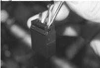
(5) Using a small flat head screwdriver release the small clips on the plug and flip the locking tab back to expose the pin connectors in the plug.
