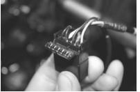
(9) Locate the wires coming from the thumb heater. Repeat step 6 to remove all thumb heater wires from the plug.
