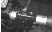
(3) Using an Alan key, undo the bolt on the clamping plate of the thumb throttle. Use a flat head screwdriver to push in the small tab while sliding the plastic clamping plate away from your grip. (Some models may have different style throttle block) You may have to take off the kill switch by removing the torx screw before taking off the throttle clamping plate.
