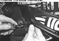
(1) Take off the side panels of your machine by undoing the latches and pulling the panels off. Using a small flat head screwdriver release the two rivet tabs on either side of the hood by prying the centers out.
