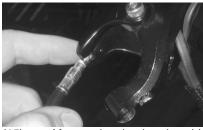
(15) After routing the throttle cable in front of the handlebars, insert the throttle cable end into the finger lever slot.
