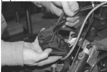
(20) Cover up the harness plugs with the cloth boot and tuck them back into the machine. Put the hood back on making sure to connect all the harness plugs that were disconnected earlier. Fasten hood bolts and rivets. Install side panels.
