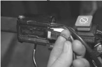
(9) Remove the throttle position switch from the throttle block and remove the throttle block from the handle bar.
