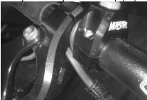
(14) Undo the two clamp bolts on your new finger throttle using an Alan key. Route the wires from the heated grip through the slot in the throttle block. Clamp the finger throttle assembly to the handle bar and snug up the clamp bolts being sure not to pinch the wires.
