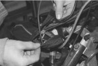
(3) Remove the black cloth cover that contains the wiring harness in front of the steering column. Undo the Velcro to expose the harness plugs.
