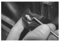
(8) Use a pick tool to remove the C-clip holding the throttle cable housing in. Pull the cable housing out and slide the cable through the slot to detach the housing.
