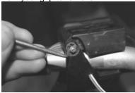
(7) Remove the pivot pin from the thumb lever by removing the E-clip and sliding the pin out. Slide the throttle cable end out of the thumb lever to detach the thumb lever from the assembly.
