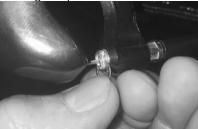
(17) Using the C-clip provided with your finger throttle, install it onto the end of the cable housing.
