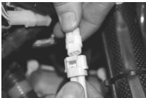
(13) Plug the white bypass connector provided with your finger throttle into the plug the throttle safety switch was disconnected from.
