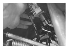
Tighten the adjuster lock nut and slide rubber boot back over the cable adjuster. Check again for proper freeplay in the lever.
