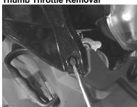
(1) Take off the side panels of your machine by undoing the latches and pulling the panels off. Using a small flat head screwdriver release the
