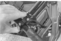
Adjust finger throttle position for rider preference and tighten clamp bolts.
