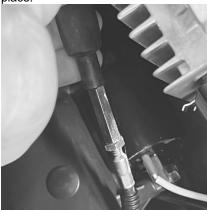
(12)Locate the throttle cable adjustment above your engine. Pull the rubber boot to expose the throttle cable adjuster. Loosen the adjuster lock nut with a wrench.
