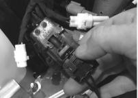
Plug your new finger throttle connector into the plug you disconnected the thumb heater from.
