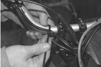
Fasten the wires with zip ties (14)to the locations previously cut. Put the dash panel, console and hood back on making sure to connect all the harness plugs that were disconnected earlier. Fasten console bolts and all plastic rivets, making sure to reconnect the air intake to the console. Install side panels.
