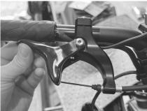
With the throttle lever in the full throttle position, tighten the cable tension by unscrewing the throttle cable adjuster until you feel the finger lever start to lift away from the handlebar. Screw the adjuster back in one full turn. The finger lever should contact against the grip firmly with no excess tension on the cable.
