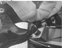
Using the C-clip provided in your finger throttle kit, install it onto the end of the cable housing to secure it in
