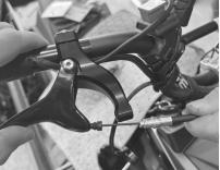
After routing the throttle cable in front of the handlebars, insert the throttle cable end into the finger lever slot. Slide the rubber seal towards the lever and pull on the cable housing to extend the cable. Slide the cable through the slot in the aluminum block and release the housing into place. Slide the rubber seal back over the
