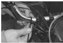
(21) Fasten the wires with zip ties to the locations you previously cut. Put the dash panel, console and hood back on making sure to connect all the harness plugs that were disconnected earlier. Fasten console bolts and all plastic rivets, making sure to reconnect the air intake to the console. Install side panels.
