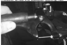
(19) With the throttle lever in the full throttle position, tighten the cable tension by unscrewing the plastic adjuster until you feel the finger lever
