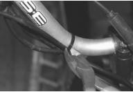
Cut the zip ties holding the wires running from the throttle block to the harness plug in the Velcro pouch.
