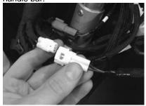
(10) Follow the wires from the throttle safety switch to the harness plug. Using your thumb, press down the lock tab to disconnect the plug connector.
