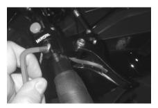
(22) Adjust finger throttle position for rider preference and tighten clamp bolts.
