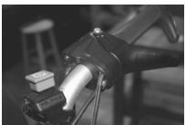
Using a Philips screwdriver, undo the four screws to remove the backing plate on your thumb throttle block.
