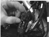
(11) Follow the wires from your thumb heater to the harness plug and disconnect the plug.
