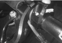
(14) Undo the two clamp bolts on your new finger throttle using an Alan key. Route the wires from the heated grip through the slot in the throttle block. Clamp the finger throttle assembly to the handle bar and snug up the clamp bolts being sure not to pinch the wires.
