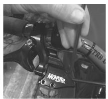
(3) Insert the two rounded mounting tabs into the sockets on the back side of your finger throttle block. Install the two 6mm bolts from the packaging of your throttle guard into the throttle guard body to fasten it to the finger throttle. Tighten the bolts so that the throttle guard body is secure, and the bolts are fully seated.
