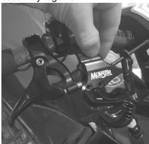
(2) Install the body of the throttle guard by sliding the throttle cable in the slot of the throttle guard body. If your machine has a throttle cable adjuster with rubber boot over it, you may have to slide the rubber boot back in order to get the cable through the slot. Alternatively, you can remove the
