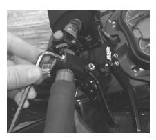
(5) Adjust the clamp bolts of your finger throttle so that your throttle assembly can rotate on the handle bar under impact. It should be snug enough so that it doesn't move around during normal operation, but you can rotate it back and forth by hand if you try hard. It is important the throttle and guard can spin easily under impact to avoid damage and accidental throttle activation if you hit a tree.
