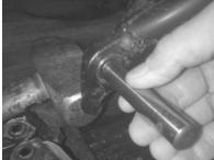
(3) Using a hammer and punch, hammer out the pressed in heim joint. You can get someone to hold a big hammer against the back side of the swing arm to take most of the impact.
