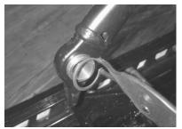
(5) Once the brass is pressed in fully, install the retaining ring included in your kit. If the retaining ring does not seat fully in the groove, the brass is most likely not pressed in fully. Repeat step 4 to get the brass fully seated.
