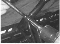
(1) Lift up and support the back of your machine so the track is slightly off the ground. Make sure the machine is stable. Remove the 8mm bolt holding your T-motion heim joint.
