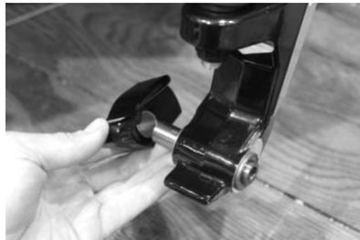
(5) Install one of your new ski bushing savers in place of the plastic spacer. The ski bushing savers can be mounted on either side of the spindle to make your ski stance wide or narrow depending on rider preference.
