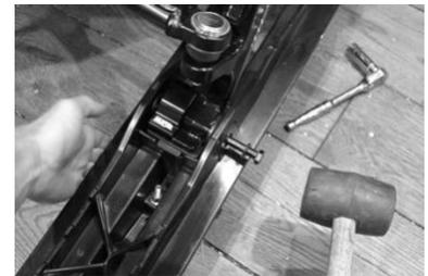
(7) Once the ski bolt is in place, install and tighten the nut.
