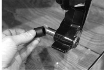
(4) Remove the plastic spacer from the sleeve.
