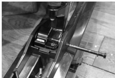
(6) Fit the ski to the spindle with your ski bushing saver in place. Angle
