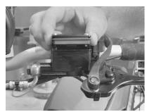
(11)Install the diaphragm and cap. Tighten down the cap bolts until you see the edge of the rubber diaphragm seal bulge only slightly. Do not overtighten, as it will squish the rubber diaphragm out of the flange and
