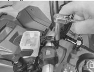
(3) Use an 8mm socket and rachet to remove the master cylinder bar clamp. Keep the master cylinder level so the fluid doesn't spill.
