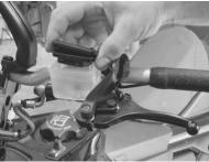
(2) Remove the cap and rubber diaphragm from the reservoir.
