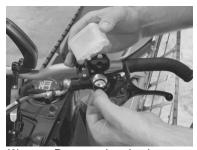
(6) Remove the plastic reservoir along with the rubber O-ring that seals it. Dispose of the O-ring. **Installation**
