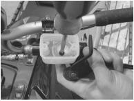
(5) Unscrew the Phillips screw inside the bottom of the reservoir.
