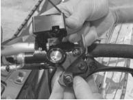
(7) Place the new O-ring included with your Munster brake reservoir into the bore of your master cylinder. Install the billet reservoir pressing it down firmly with your thumb. Make sure the reservoir is fully seated in the O-ring before proceeding to the next step.
