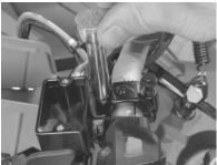
(8) Install the master cylinder bar clamp, making sure the arrow is pointing to the back of your snowmobile. (Backwards from how it came stock) Tighten down only the bolt closest to the reservoir until its snug, making sure your reservoir is level.
