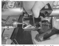
(9) Install and tighten the Allan screw included with your Munster brake reservoir. Only tighten it with the long end of an Allan key until it bottoms out, making sure the reservoir is fully seated. DO NOT OVERTIGHTEN OR IT MAY STRIP THE THREADS IN YOUR MASTER CYLINDER WHEN YOU GO TO REMOVE IT.
