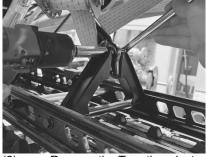
(2) Remove the T-motion pivot bolt from the top of the pivot arm
