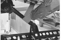
(1) Suspend the rear of your snowmobile so the skid and track are hanging freely. Using a rachet strap, loop the strap over your tunnel and around your rear swing arm. Tighten the strap to compress your suspension slightly. The objective is to remove any preload your suspension is putting on the pivot arm in order to remove the pivot bolt.
