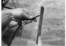
(5) Remove the steel sleeve from the OEM pivot arm and clean the grease off with a rag. Use a flat file to file the edges of the sleeve and remove any burs or flare that might exist from it being installed. Sometimes the sleeve can be mushroomed slightly at the ends preventing it from sliding into the Munster pivot arm. This material must be removed by a file in order to install the sleeve.
