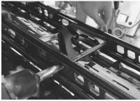
(3) Remove the lower pivot bolt, making sure not to lose the two washers in between the rails and the pivot arm.
