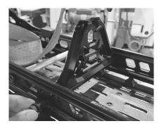
(7) Install the pivot arm on the machine, making sure the two washers are in place between each side of the sleeve and the rails. Once the bolt and washers are in place, install the nut and tighten to 27 ft-lbs.
