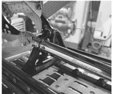
(9) Install the top pivot bolt included with the Munster pivot arm into the T-motion join. Thread the bolt into the locknut and tighten to 27 ft-lbs. Remove the rachet strap compressing your suspension.
