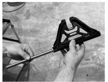
(6) Install the sleeve into the Munster pivot arm.
