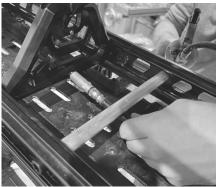
(10) Grease the lower grease fitting on your pivot arm with waterproof grease, according to grease specifications from your BRP manual.
