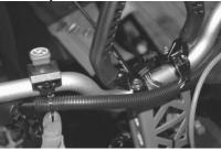
(2) Take off the riser cover to expose the wiring harness plugs. Follow the wires from the kill switch to the wiring harness, cutting the zip ties to expose the wires. Unplug the harness plug that the wires go to.
