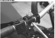
Unscrew the small torx screw to remove the stock kill switch assembly.
