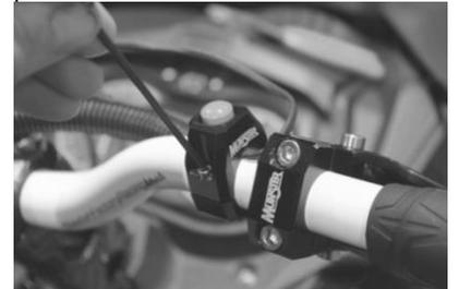
(7) Remove the clamp from the Munster kill switch with an Alan key. Install the kill switch on the handle bar in your desired position, routing the wires appropriately.
