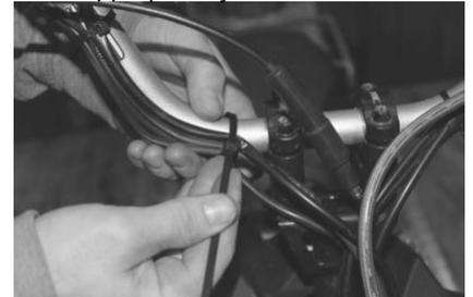
(8) Use zip ties to fasten the kill switch wires to the handle bar and you're done!
