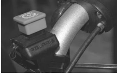
(1) Unscrew the two torx screws to remove the bottom clamp on the stock kill switch assembly. Remove the kill switch and cut any zip ties fastening the wires to the handle bar and riser.
