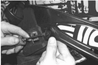
(3) Take off both side panels of your machine. Using a small flat head screwdriver release the two rivet tabs on either side of the hood by prying the centers out. Slide the hood forward to release it. Undo all wire harness plugs connected to the hood to properly remove the hood from the machine.
