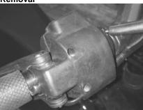
(13) With a torx screw driver remove the 4 screws from the back of the throttle assembly.
