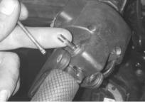
(15) Remove the pivot pin and sleeve from the throttle block. The throttle assembly should now split apart from the handle bar.
