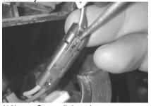
(18) Once all the wires are exposed, disconnect the plug connector to your kill switch. If you are installing a Munster reverse switch, disconnect the plug connector to the reverse switch as well. (See reverse switch instructions for pictures and further information)
