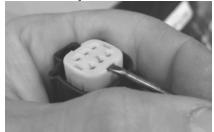
(7) Release the locking tabs holding the front cap on and pull the cap out until it stops. A second set of locking tabs prevent the cap from coming off. Pry back the second set of locking tabs to remove the cap completely. You should now be able to see all the tabs holding each terminal in and pry them back to remove them. Pull the wires through the rubber seal and backing plate of the plug connector.
