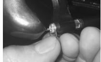
(13) Using the low profile C-clip provided with your finger throttle, install it over the end of the cable housing to secure it in place.
