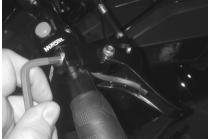
Undo the clamp bolts on the (10)Munster finger throttle using an Alan key. Route the wires from the heated arip through the open slot in the throttle block and clamp the finger throttle assembly to the handle bar. Re-route your throttle cable in front of your riser and handle bars. THE THROTTLE CABLE MUST BE AWAY FROM ANY PINCH POINTS. CHECK YOUR STEERING FOR FULL RANGE OF MOTION, MAKING SURE THERE IS NO STRESS OR TENSION ON THE CABLE HOUSING AT ANY POINT.
