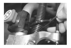
(16) Adjust and tighten kill switch if it was loosened. Route all heater and kill switch wires back in the harness and use zip ties to secure to the handle bar and riser.
