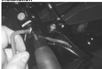
(6) Undo the two clamp bolts on the new finger throttle using an Alan
