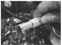
(5) Remove the hood and follow the wires from your thumb throttle to the beige connector above the engine. Disconnect the connector by pressing on the release tab. This connector will remain unplugged.
