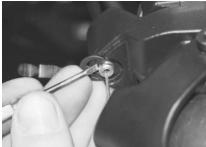
(1) Remove the C-clip holding the cable housing in place. Pull the cable housing out from the throttle assembly, and remove the cable end from the thumb lever. Re-route the throttle cable in front of the handle
