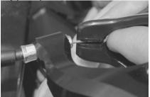
(8) Insert the ball end of the throttle cable into the socket of the
