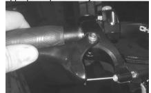
(10) Locate the throttle cable adjuster. With one hand pulling the throttle lever to the bar, tighten the cable by unscrewing the cable adjuster until you feel the lever start to pull away from the handle bar grip. Screw
