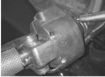
(12) With a torx screw driver remove the 4 screws from the back of the throttle assembly.
