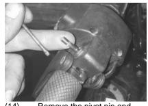
(14) Remove the pivot pin and sleeve from the throttle block. The throttle assembly should now split apart from the handle bar.
