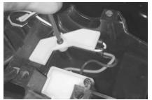
(16) With a small torx bit, remove the screw in the white plastic retainer holding all the wires in the throttle assembly.
