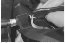
(20) Insert the ball end of the throttle cable into the socket of the lever. Pull on the throttle lever to make sure the cable ball end is seated and rotates freely.
