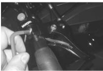
(18) Undo the two clamp bolts on the new finger throttle using an Alan key. Route the wires from the heated grip through the slot in the throttle block and clamp the finger throttle assembly to the handle bar.
