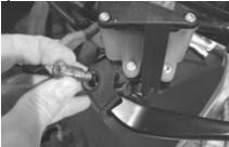
Slide the pivot bolt out from the assembly and remove the rubber boot and brake lever.
