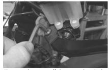
Loosen off the torx pivot bolt on the stock brake lever, but do not remove it yet from the assembly
